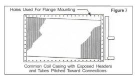
From a coil casing standpoint, the only difference between these designs is that the flange mounted coil requires holes around the perimeter of the case flange. To simplify matters, many coil manufacturers provide holes on all coil casings. The headers on these case designs may be exposed or enclosed depending on the manufacturer and, to some extent, the coil type
