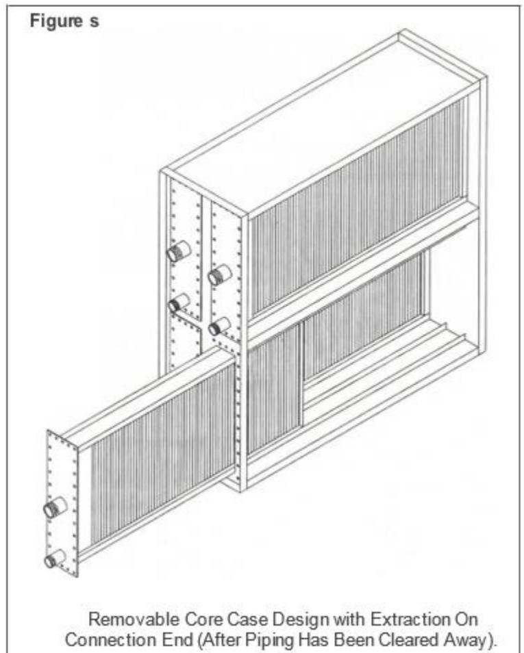
Depending on the manufacturer, single or multiple cores can be provided in the same housing. The housing can be designed to accommodate multiple coils across the face and/or multiple coils in depth. The coils and housing can be orientated for horizontal or vertical air flows.
