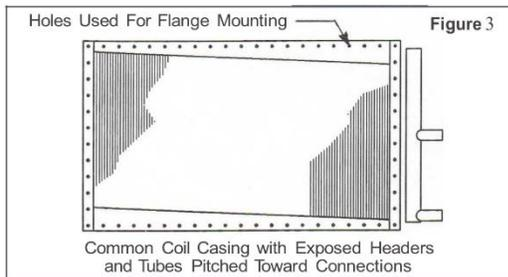
From a coil casing standpoint, the only difference between these designs is that the flange mounted coil requires holes around the perimeter of the case flange. To simplify matters, many coil manufacturers provide holes on all coil casings. The headers on these case designs may be exposed or enclosed depending on the manufacturer and, to some extent, the coil type
